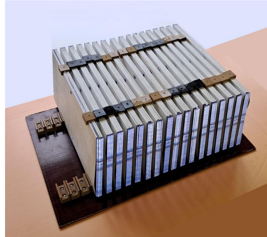
Calorimeter with 310x190 mm scintillators
